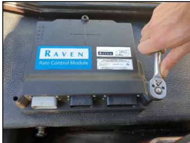
FIGURE 16. RCM - Sprayer ECU Cable Connections
