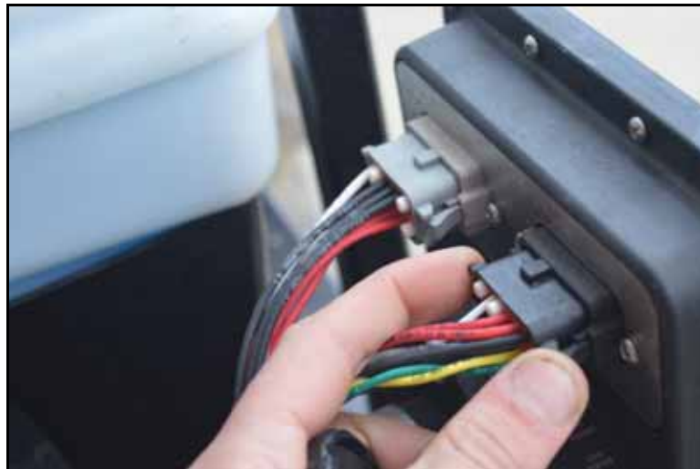
FIGURE 17. Sidekick Pro™ ICD Pump Connections
