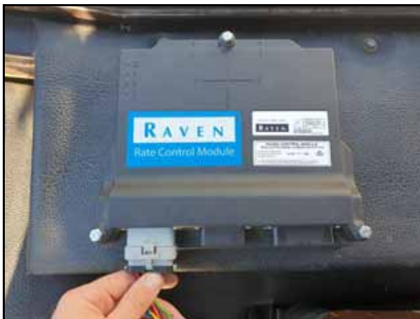
FIGURE 16. RCM - Sprayer ECU Cable Connections
