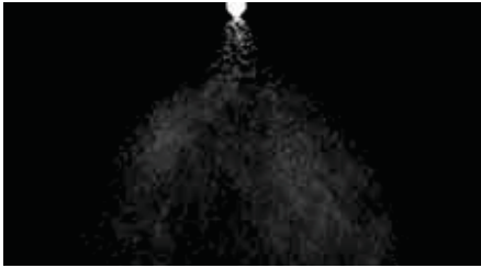
80° or 110° wide spray patterns; broad flow range and droplet spectrum to fit many spraying applications.
