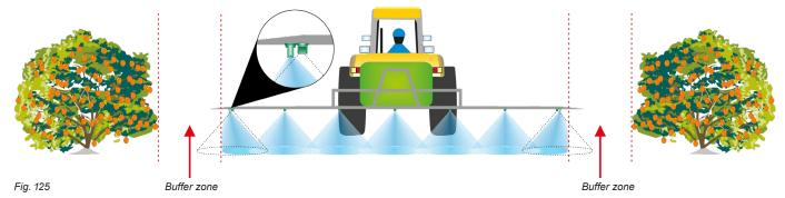
If this function is enabled under implement basic settings (chap. 10) it is possible to alternatively select standard or special nozzles. Nozzle selection modes are variable (they vary based on the Auxiliary Input connected to the VT). Following are some examples.
