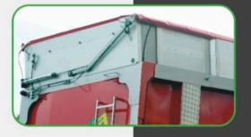
Lateral PVC cover with pneumatic arms Rapid release system ideal for wood chips pneumatically operated with hard structure
