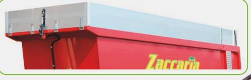
On demand: Aluminium extension side and hydraulic opening of the front extension side.
