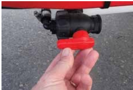
Figur 15: Kugleventil i sugeposition
